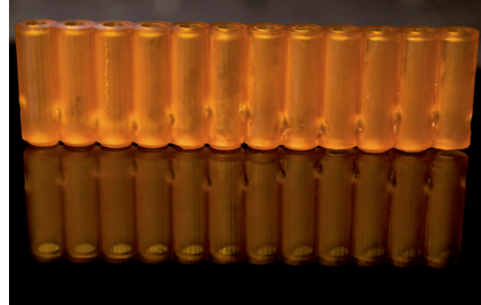
► Acoustic lattice with sinusoidal connections for sound trapping
