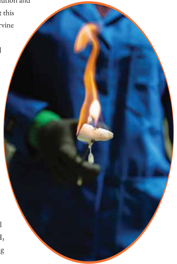
Figure 1 ▲ A burning snowball. Water drips during methane hydrate combustion
